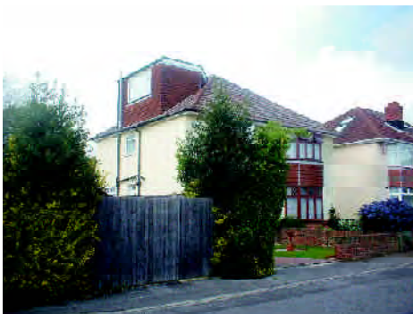
Dormer windows should not dominate the main roof form, nor should they be higher than the ridge of the main roof
