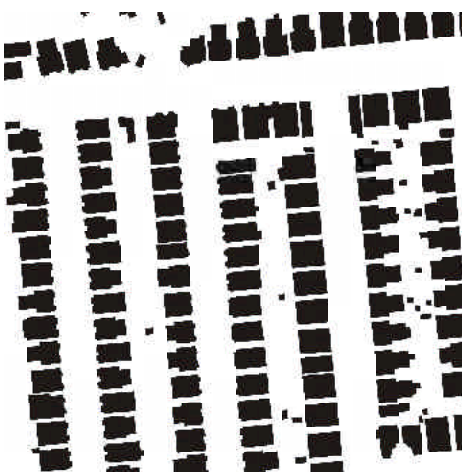
A figure-ground study shows the density of development (74dph) in proportion to the private space and public realm
